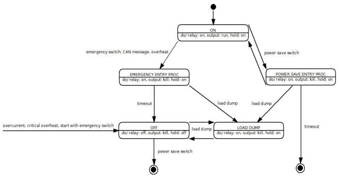
The device operation can be best explained with state machine diagram:
